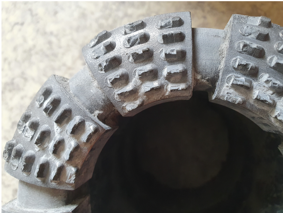
Fig. 3-4: Synset core bit after POOH from a depth of 271 m MD
