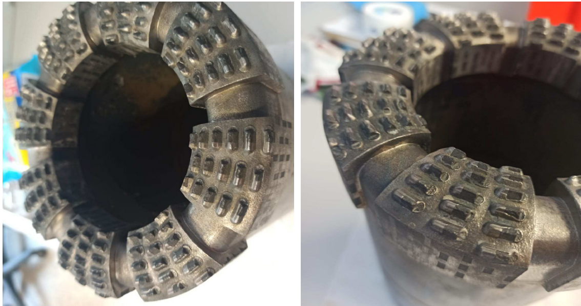
Fig. 3-6: Synset core bit after POOH from a depth of 615 m MD
