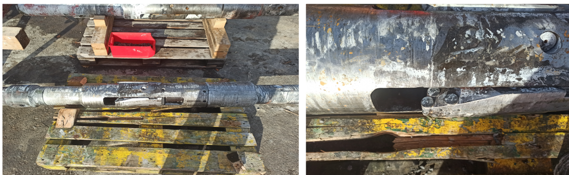
Fig. 3-8: 9 \frac{7}{8} " underreamer with malfunctioning hydraulic arms after POOH
