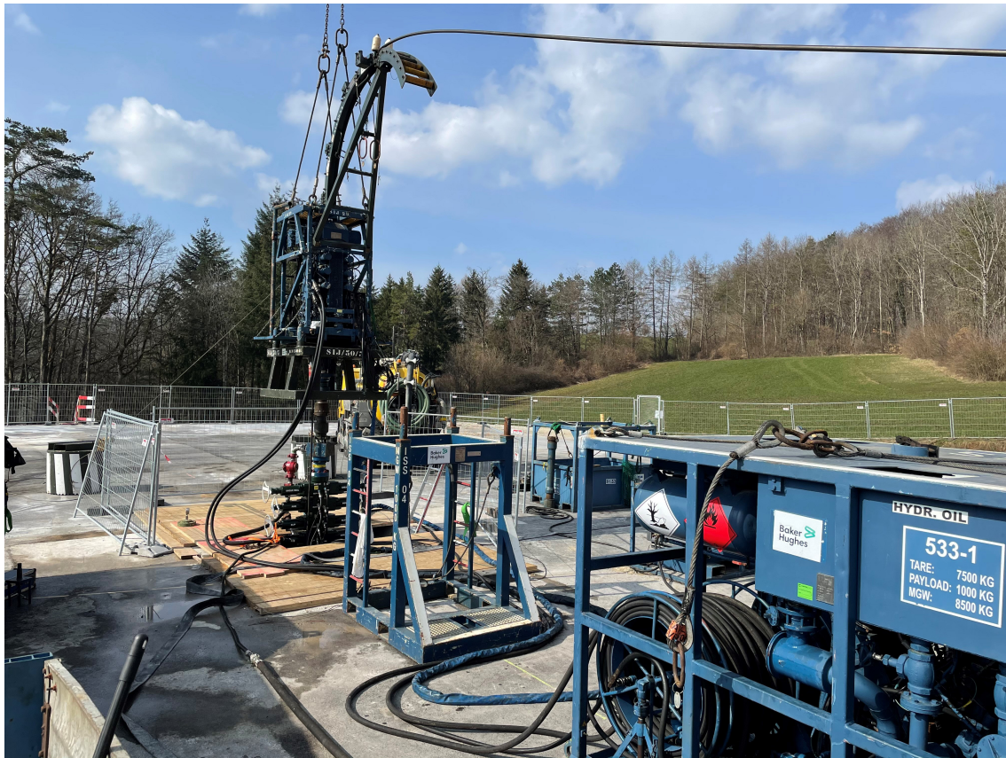
Fig. 3-15: Coiled tubing operation during RIH
