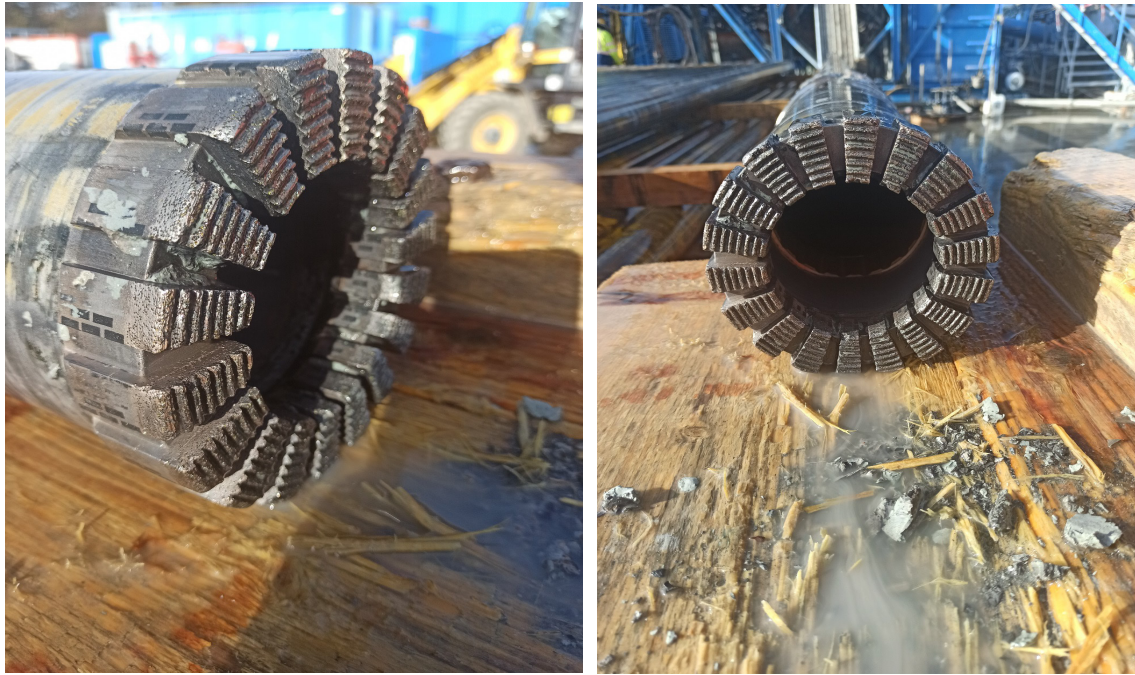
Fig. 3-11: Impregnated core bit after POOH from a depth of 658 m MD
