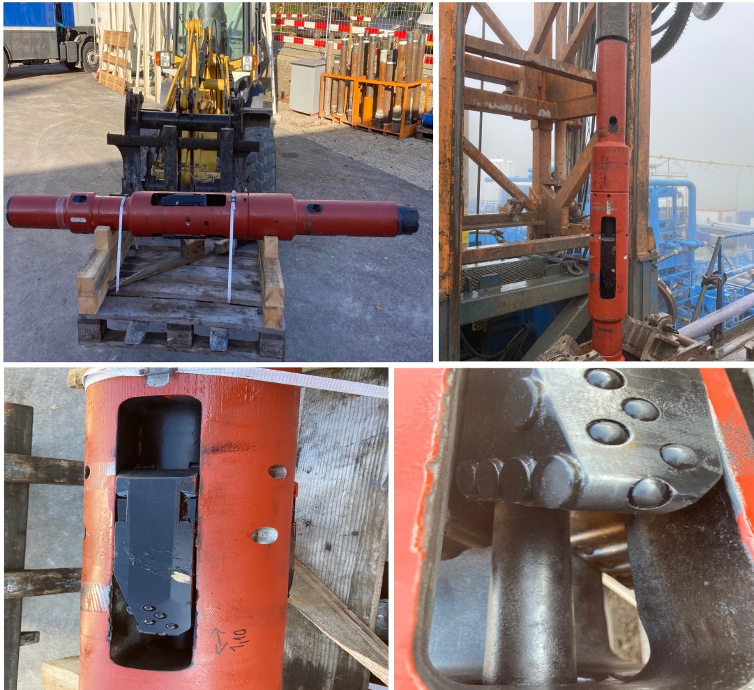
Fig. 3-7: 9 \frac{7}{8} " underreamer before RIH
