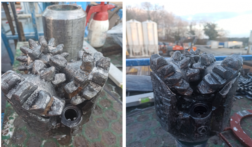
Fig. 3-9: 6 \frac{1}{2} " tricone bit after POOH
