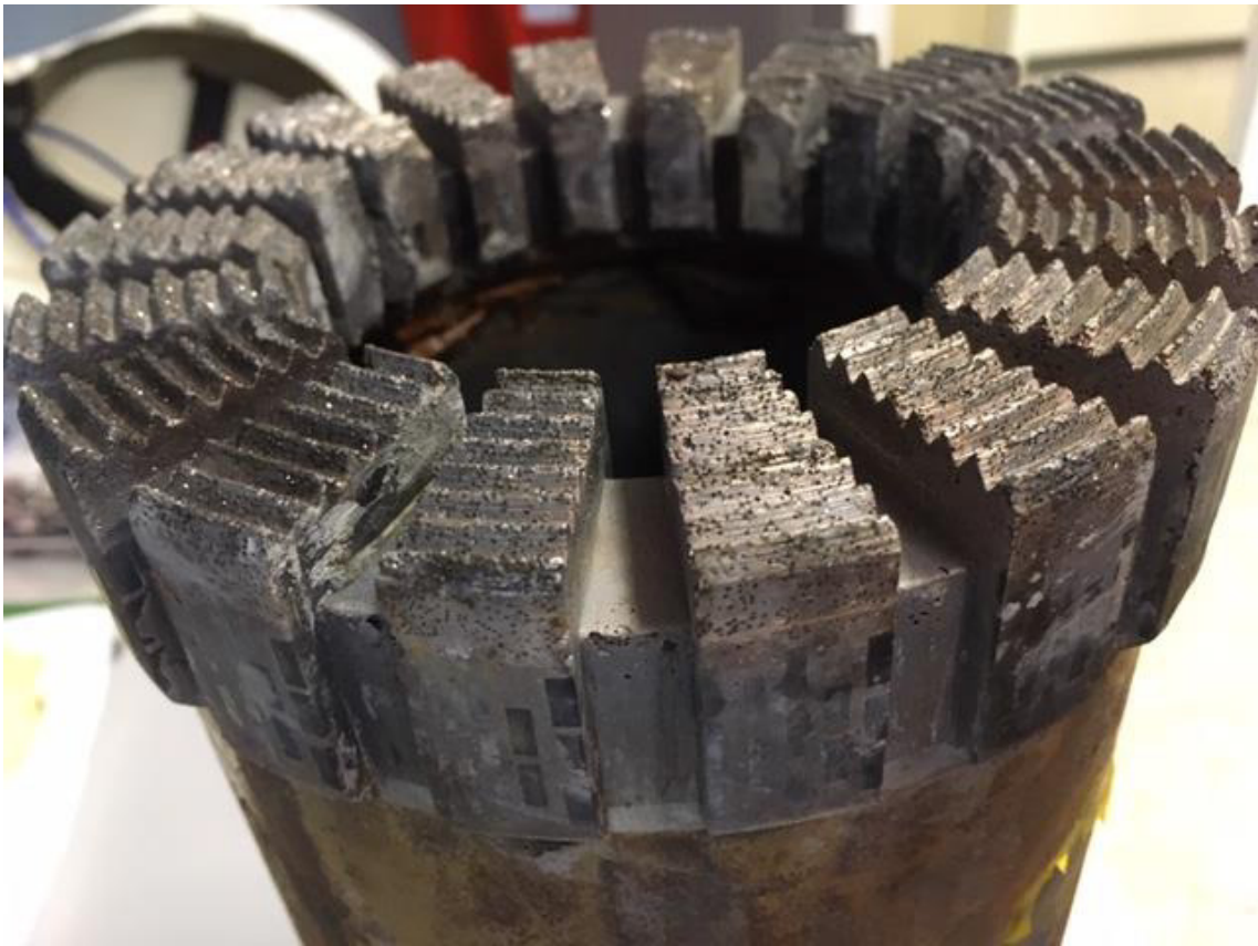
Fig. 3-5: Impregnated core bit after POOH from a depth of 370 m MD
