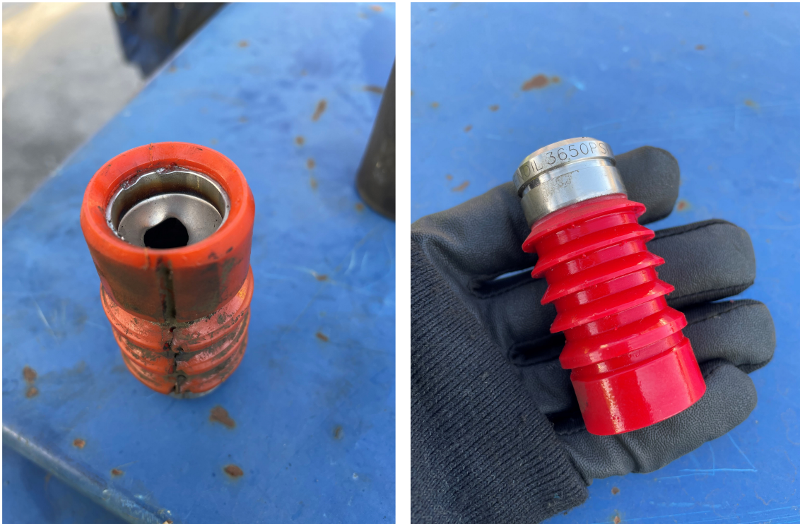
Fig. 3-16: First dart after recovery (left) and second dart that could not be recovered (right)
