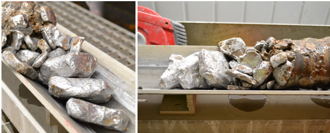
Fig. 3-10: Aluminium parts from the 7 \frac{5}{8} " casing shoe recovered from a depth of 617 m MD in the first core of Section III
